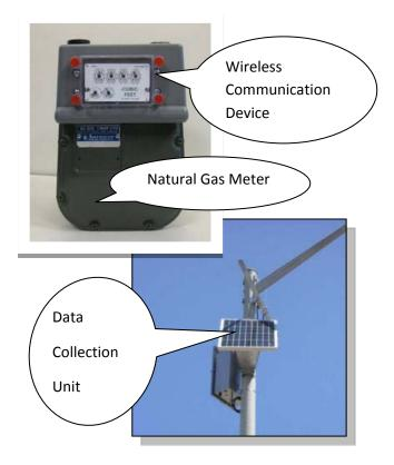
Gas usage is still recorded in the traditional way, but with the new wireless communication device, it becomes an "advanced meter" that securely and electronically transmits hourly natural gas usage reads every six hours to data collection units, which then securely forward the information to SoCalGas. Customers will have access to their hourly natural gas usage information on a "next-day" (or sooner) basis.
