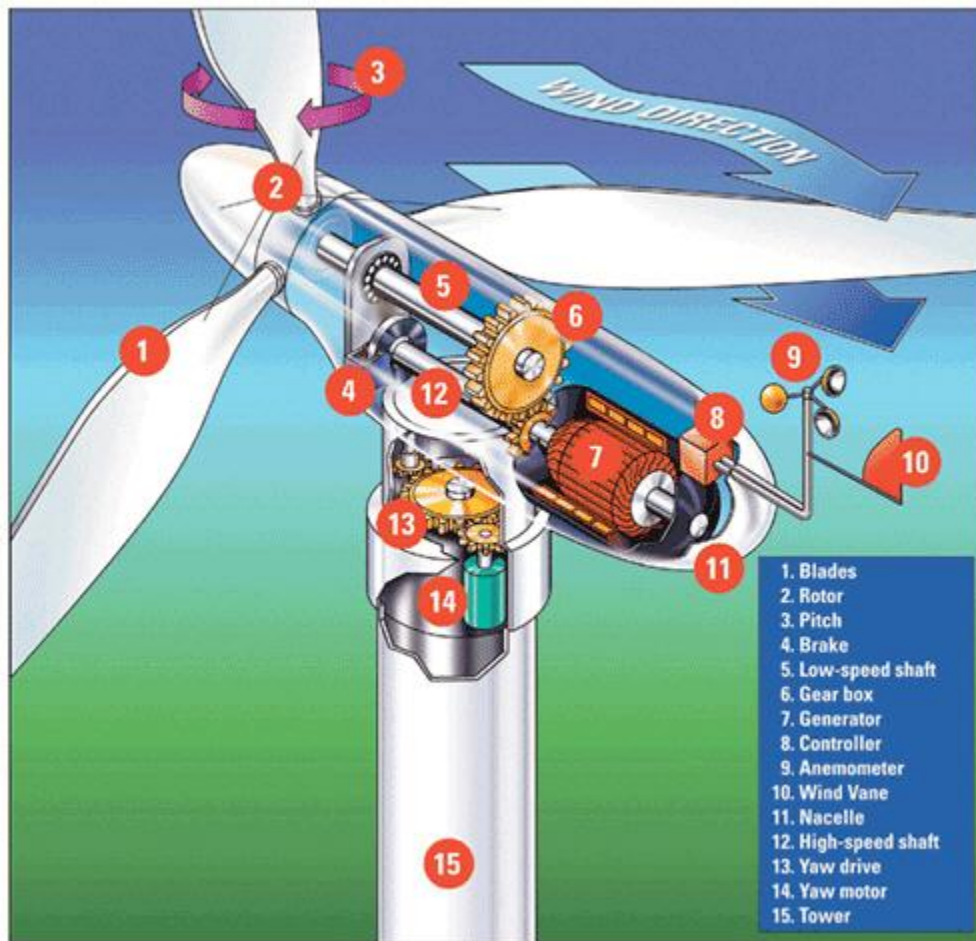
Figure A-38: Wind Turbine Components
