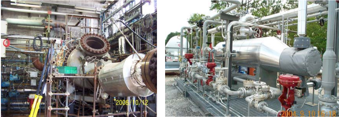
Figure 3: Test rig & mixing skid setup during LNG testing
