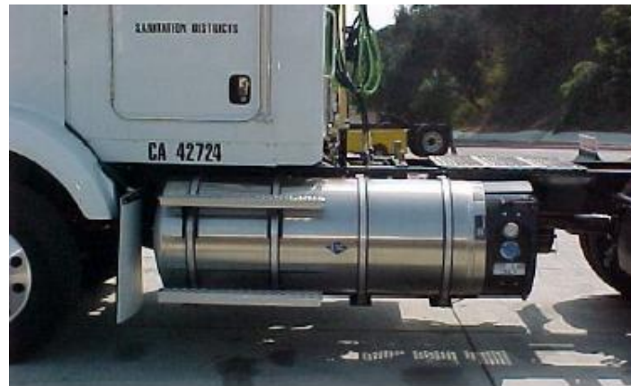
A 120-gallon LNG tank is mounted under the cab.
