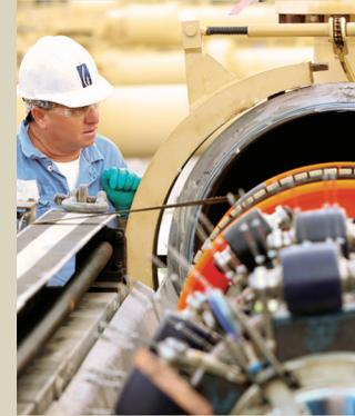
We use advanced safety inspection tools to determine pipe condition and help ensure that the pipelines are being maintained safely.
