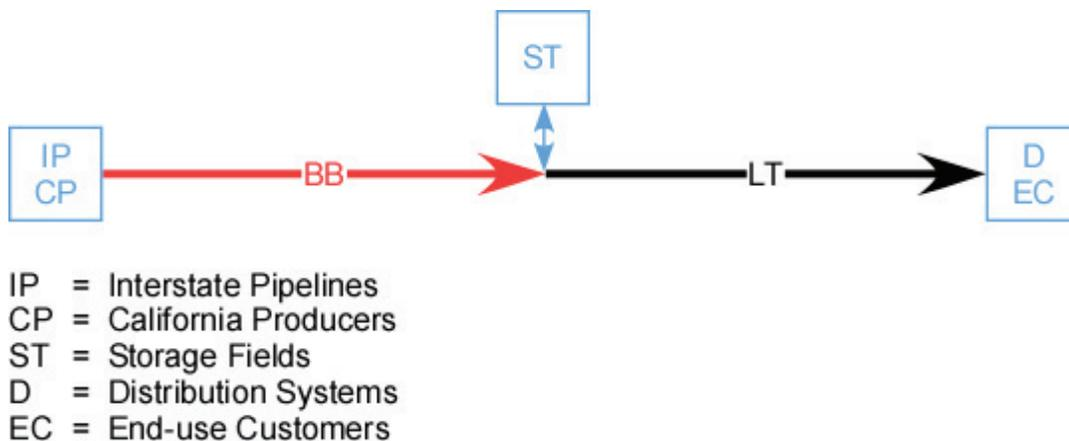
23 In Figure 3, gas supply is received from interstate pipelines and California producers, and
