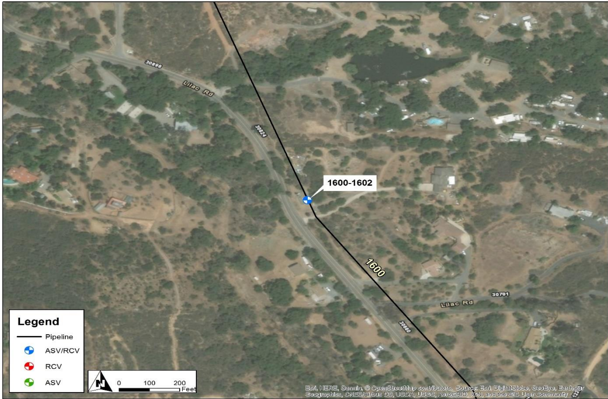
Figure 3: Satellite Image of Valve 1602
