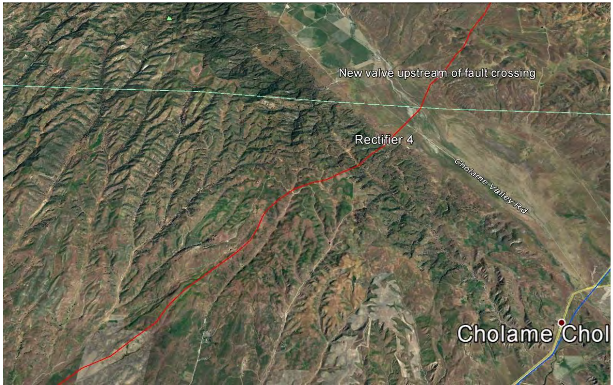
Figure 21 – Morro Bay Gas Pipeline System – Fault Broad View
