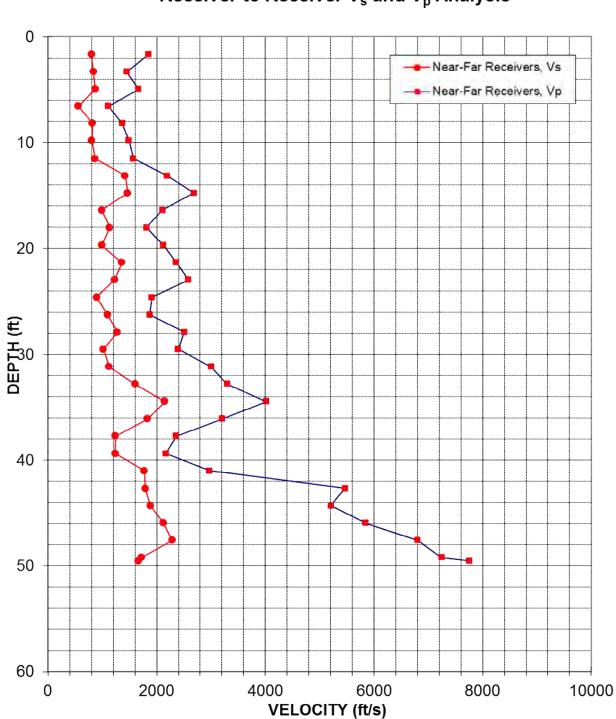
SCG BOREHOLE VCU-7 Receiver to Receiver V<sub>s</sub> and V<sub>p</sub> Analysis
