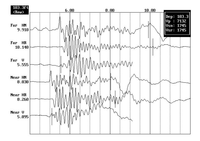
Figure 3. Example of unfiltered suspension record
