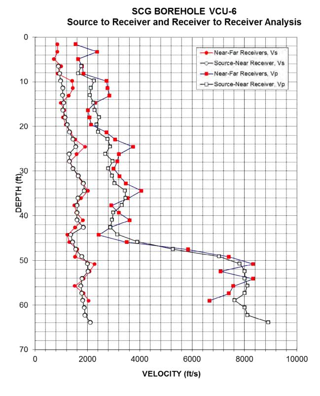
Figure A-1: Borehole VCU-6, Suspension S-R1 P- and S<sub>H</sub>-wave velocities
