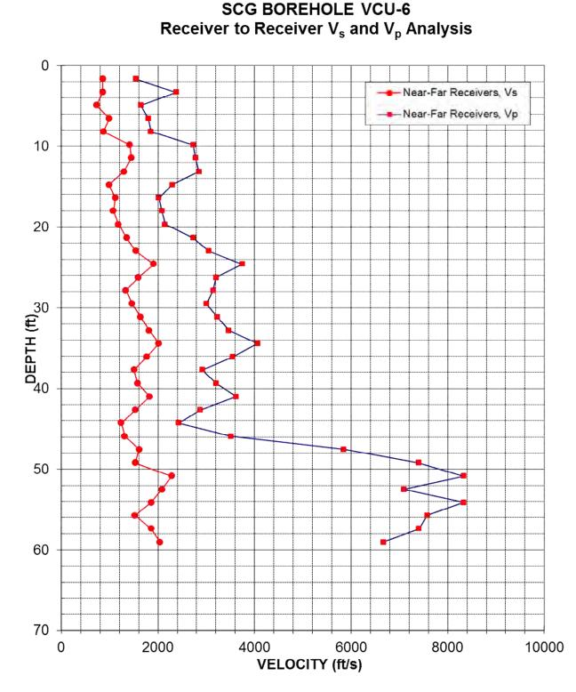
Figure 4: Borehole VCU-6, Suspension R1-R2 P- and S<sub>H</sub>-wave velocities
