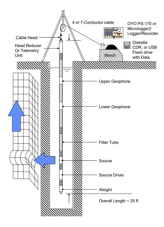
Figure 1: Concept illustration of P-S logging system
