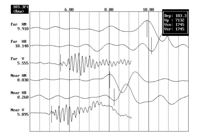
Figure 2: Example of filtered (1400 Hz lowpass) suspension record
