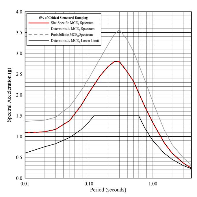
NOTES: Probabilistic  $MCE_R$  spectrum was computed for a ground motion level expected to achieve a 1% probability of collapse within a 50 year period.
