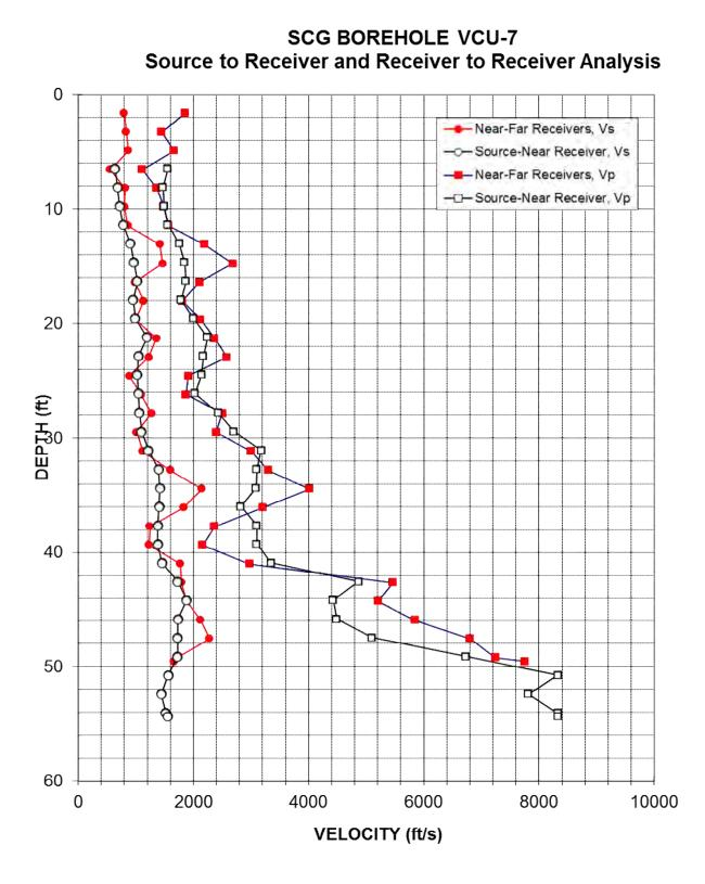
Figure A-2: Borehole VCU-7, Suspension S-R1 P- and S<sub>H</sub>-wave velocities
