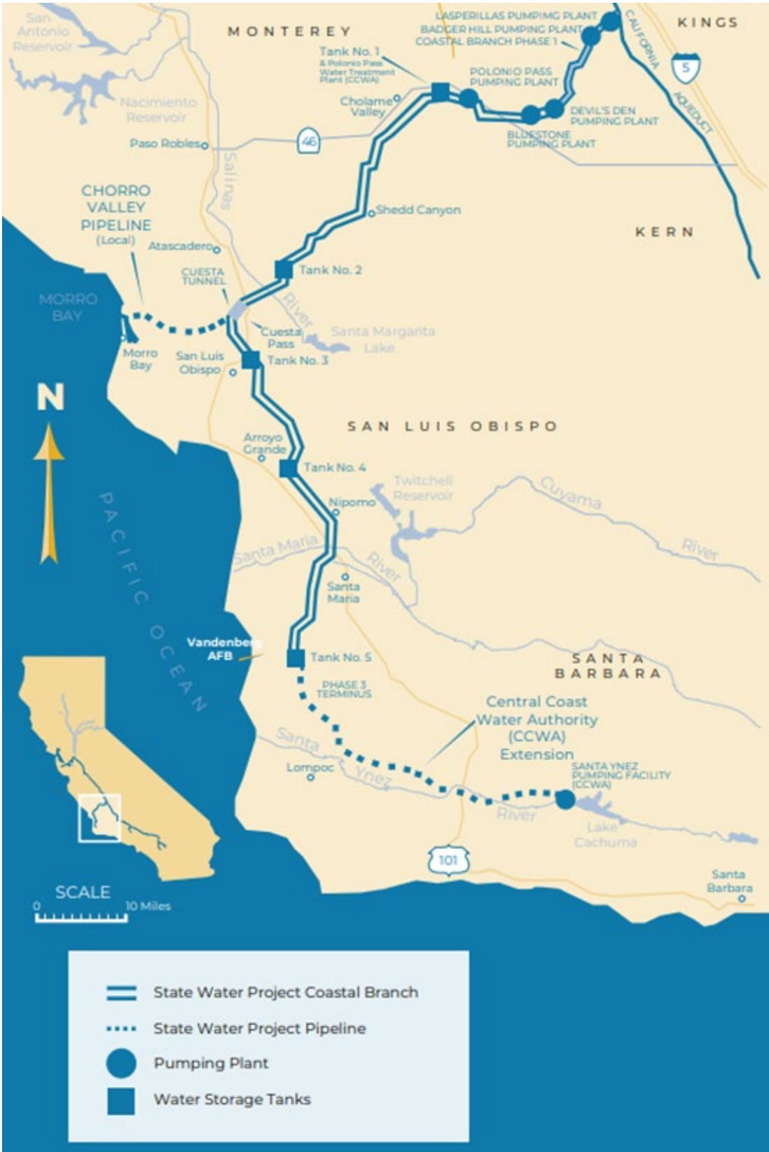
Figure 1-6 SWP Facilities – CA Aqueduct Coastal Branch
