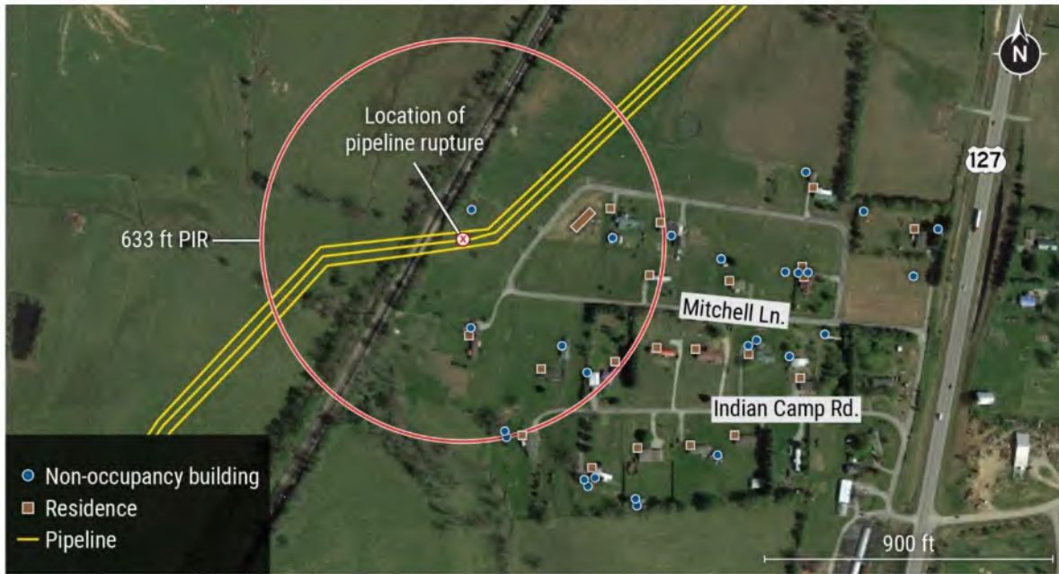
Figure 11. Human-occupancy buildings within the potential impact radius. (Courtesy of Enbridge.)
