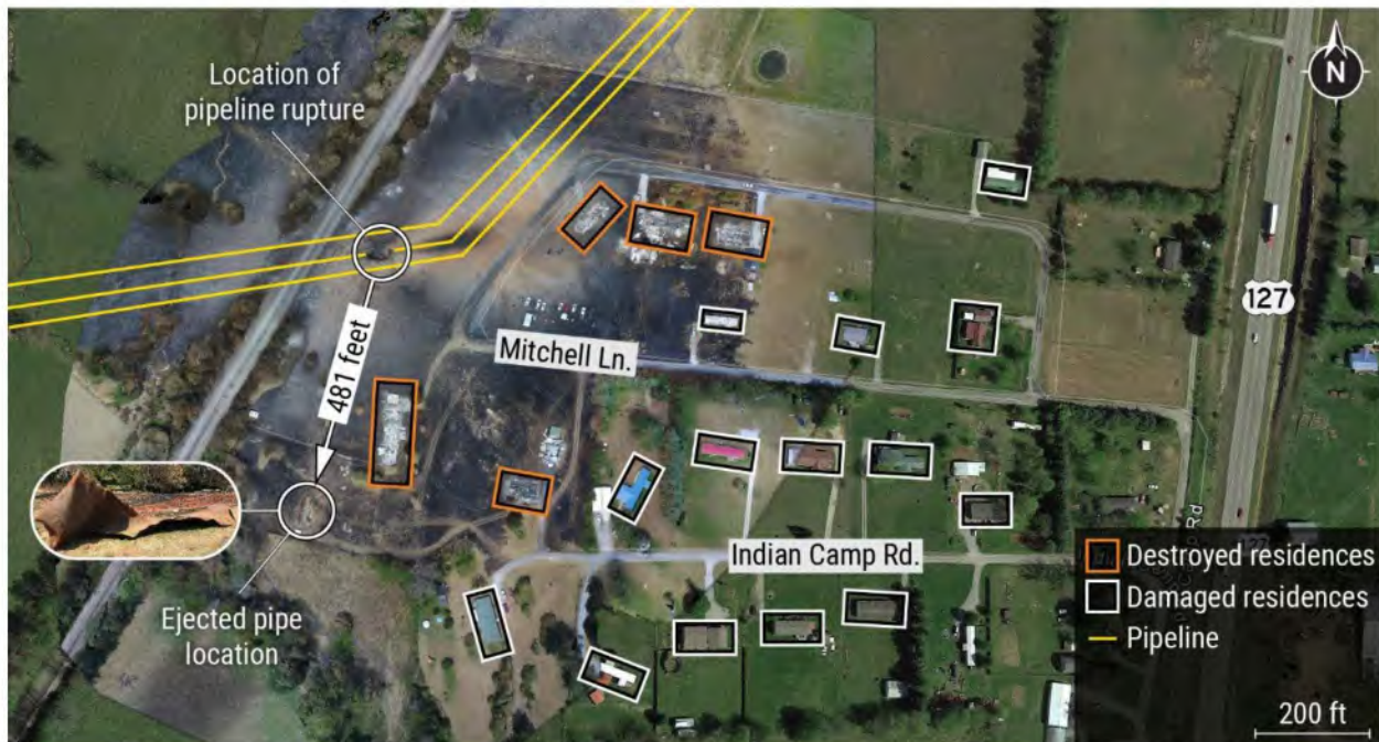
Figure 1. Aerial view of the Indian Camp Subdivision overlaid on Google Earth image.
