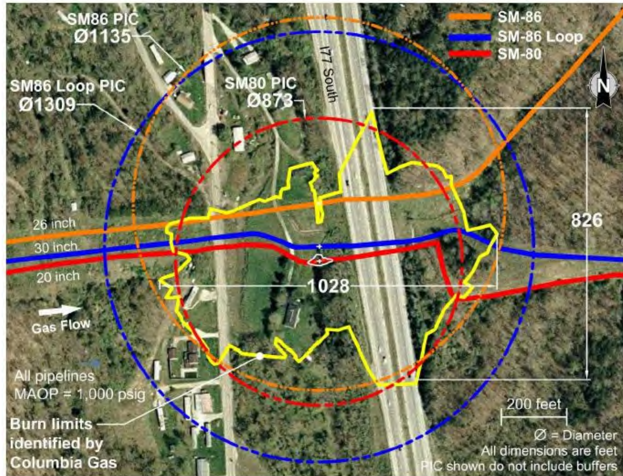
Figure 11. Potential impact radius circles for each pipeline in SM-80 system at rupture location.
