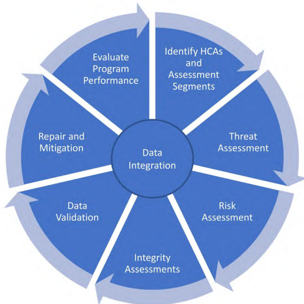
Figure 10. Integrity management process flow.
