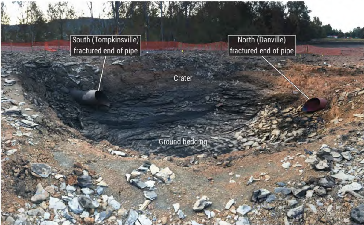
Figure 4. Crater and ground bedding at rupture site.
