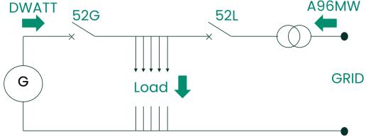
The algorithm can manage #1 Analog Signal 4-20mA from field to acquire Grid Imported Power A96MW
