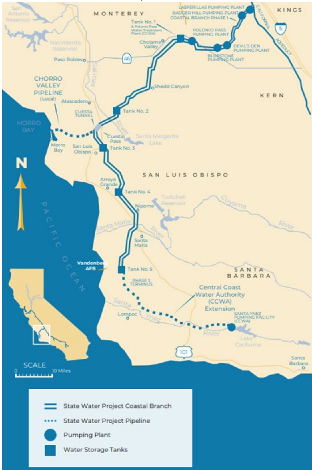
Figure 1-6 SWP Facilities – CA Aqueduct Coastal Branch
